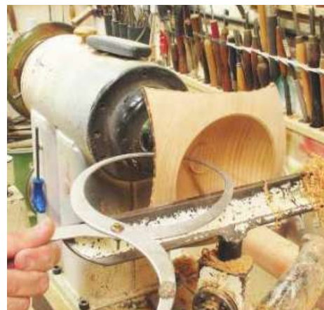
▲ Pic.30 Take the wall thickness down to a fairly even 5mm. Using hour glass callipers will allow you to measure this easily as they basically repeat on the end nearest you the thickness of the bowl
